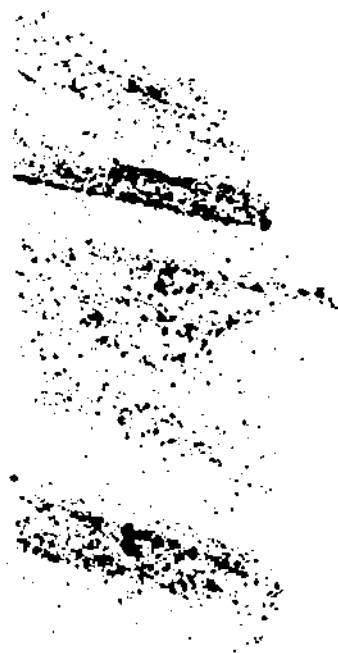
Fig.2 Activation beta-autoradiogram, fixing gold distribution in banded pyrite ore with banded disperse gold distribution (1-10 mkm).
