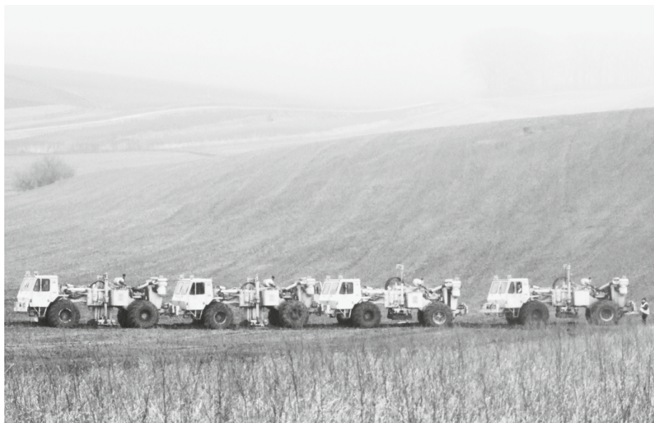
2D seismic measurement by the help of four seismic vibrators near Némčice, Czech Republic.
