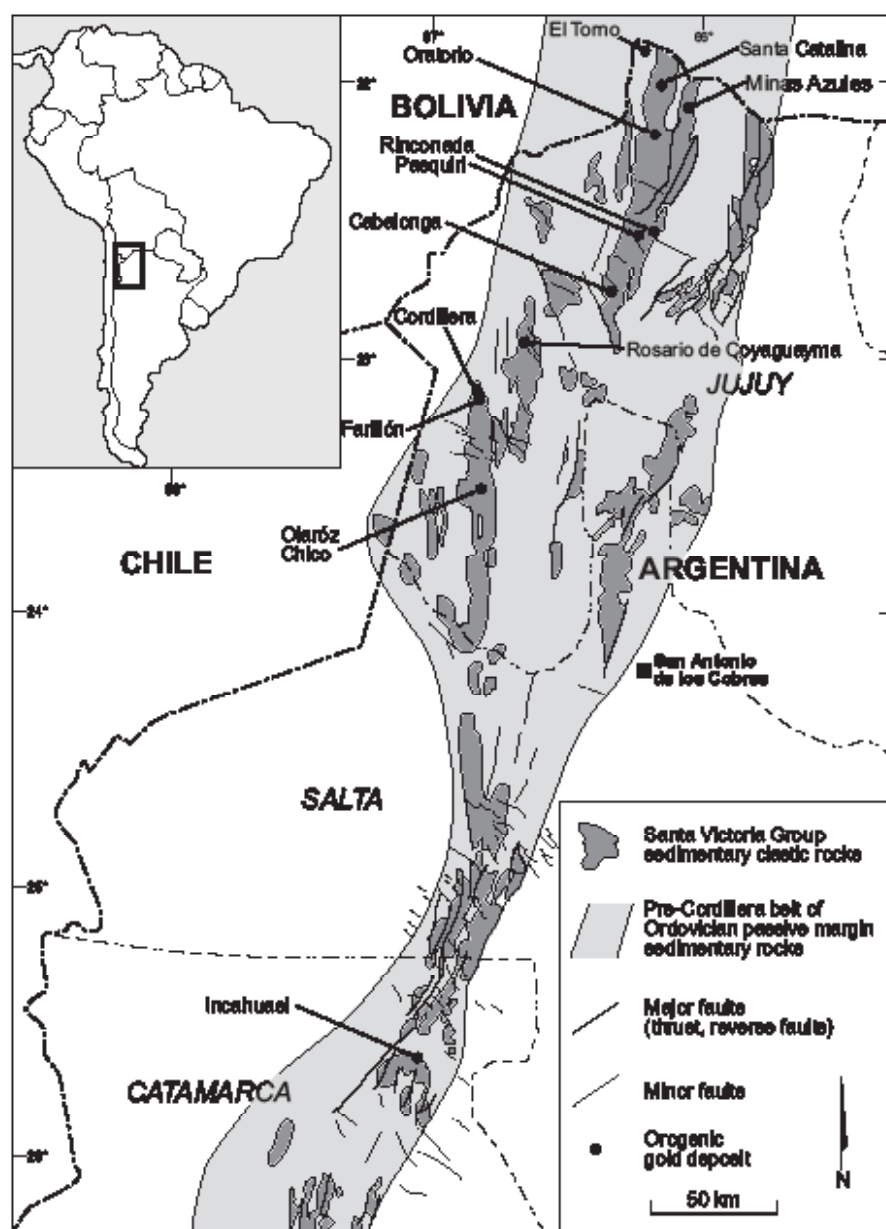
Figure 7: Distribution of the Ordovician Santa Victoria Group sedimentary rocks in the north-western part of Argentina, which host turbidite-hosted orogenic gold style mineralization. The Incahuasi deposit is located in the northern part of the Catamarca province (map modified from Cardero Resources).
