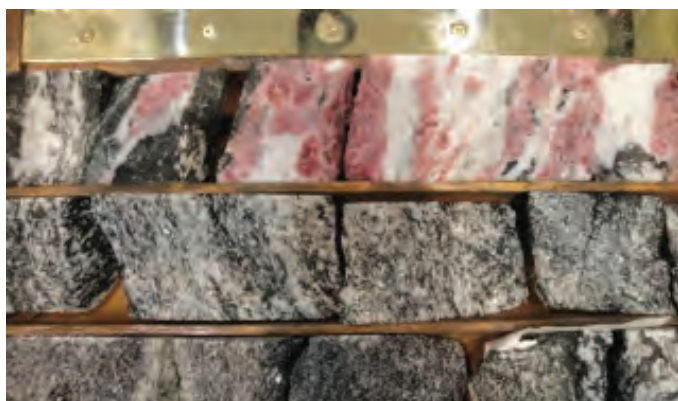
Figure 6: Occurrence of eudialyte (pink in color) [Na_{15}Ca_6(Fe,Mn)_3Zr_3(Si,Nb)(Si_{25}O_{73})(O,OH,H_2O)_3(Cl,OH)_2] in the drilled core from the Kipawa deposit in Canada.
