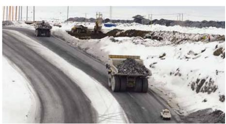
Figure 6: First Quantum Mineral/Boliden Kevitsa, gigantic Caterpillar 795F carrying 350 tons of rock, followed by a pick-up (for the scale).
