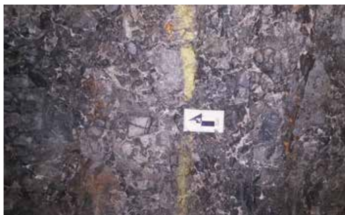
Fig. 2: Breccia with basalt clasts and a calcite matrix, Miraflores Mine
