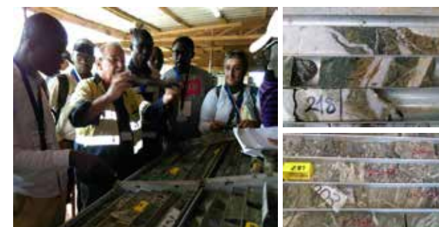
Fig. 5: Study of Perseus drill cores. Ghislain Tourigny explains alteration zones, the minerals, which are vectoring gold mineralization as well as barren and fertile facies.
