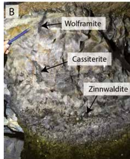
Fig. 5: (A) Coarse-grained zinnwaldite + quartz vein with surrounding massive greisen alteration; (B) Wolframite and cassiterite with quartz and zinnwaldite in one of the greisen veins (Tiefer Bünaul Stollen, Zinnwald).
