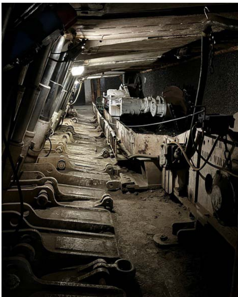
Fig. 5 Longwall shearer and hydraulic roof support in the historical „Guido” mine, Silesia, Poland
