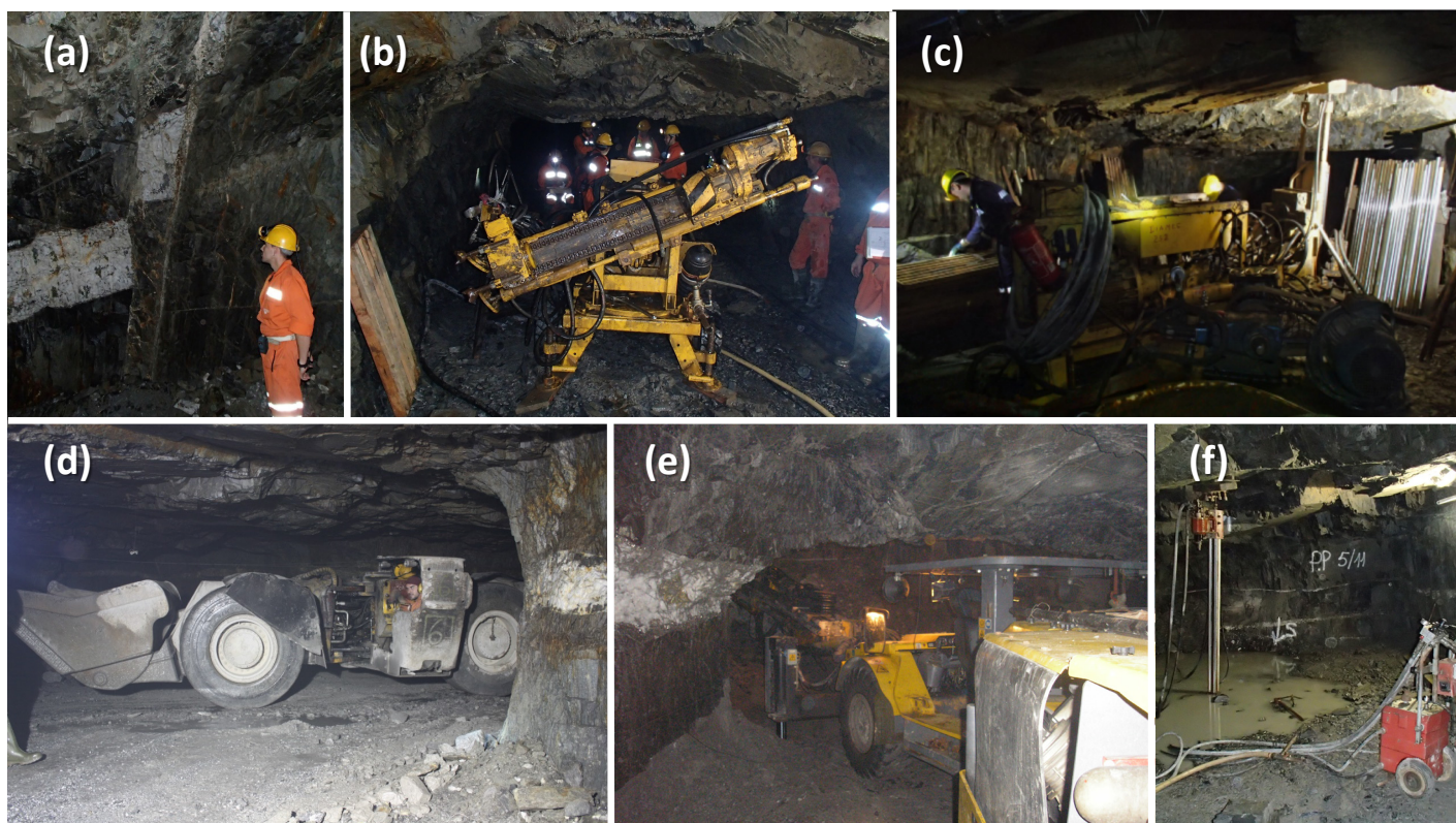
Figure 6: Modern underground works at Panasqueira – (a) the spatial continuity of the lodes as a permanent challenge, both due to the original (irregular-)lenticiform shape and common fault-related detachments; (b, c, f) planning and execution of exploration/evaluation drillings in active fronts; (d, e) general views of the mechanized room and pillar method.
