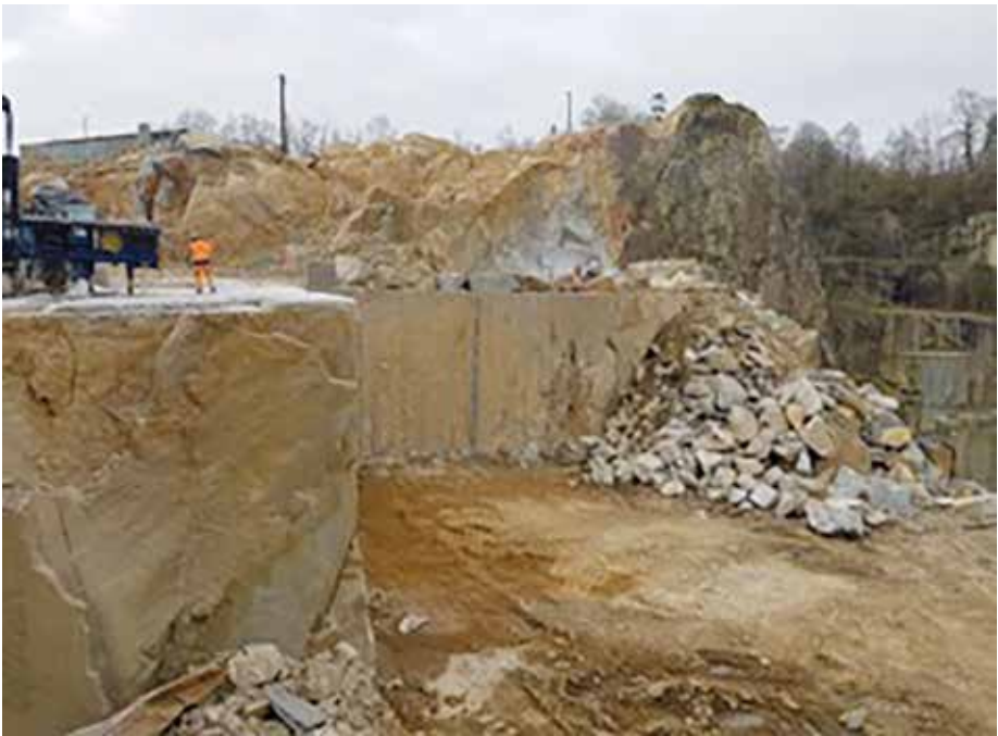
Fig. 8 Blocks of granite are being cut (La Chauffetière Quarry)
